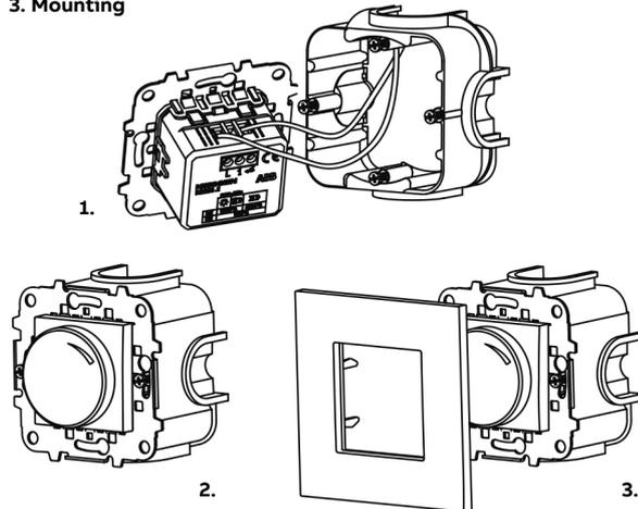
Turn the device in the correct installation position. The marks on the back side of the device, orient the correct top position.
