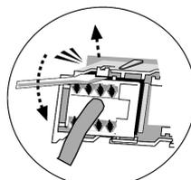
5.3 Pry downwards to release the lower hook.
