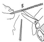
1.4 Cut the mesh (if it has one and the cord at the same level of the jacket).
