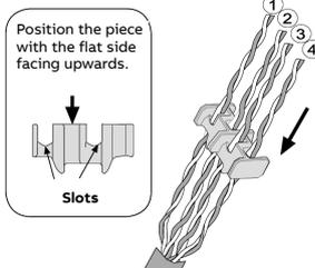
2.3 Ensure the end piece is located as close as possible to the edge of the jacket.
