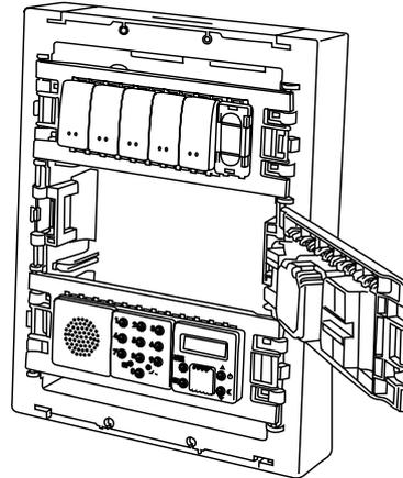
5. The mounting plate is closed by clipping.
