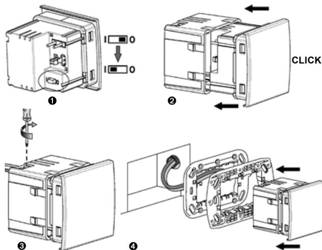
1. Move the selector from the storage position (O) to the operating position (I)
