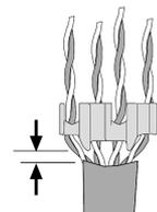
2.4 Place the pairs in the direction of the end piece slots.
