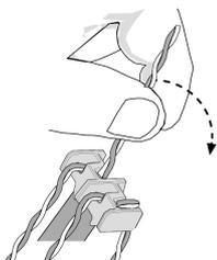
2.5 Insert the end piece into the module.
