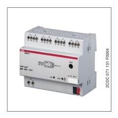
The DALI gateway is a DIN rail mounted device for insertion in the distribution board on a DIN rail. It is used to control DALI devices e.g. electronic ballasts, transformers, relays etc. via the EIB/KNX.
