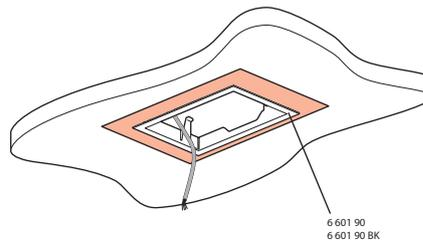
This accessory is only installed with flush-mounting frame 6 601 90, 6 601 90BK and URA NEXT self-contained emergency lighting units.
