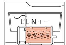
TELEC - Connection terminals: direction of connection with Legrand remote control Cat. No. 0 039 00 must be complied with.
