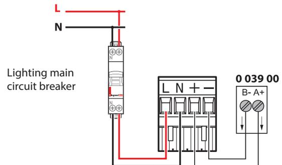
**Note:** Although self-contained emergency lighting units do not consume much power, you must check that the line dedicated to these lighting units can deliver the necessary current. You will find below the current the line needs to withstand for 100 installed lighting units according to the catalogue number (for simplicity, we have assumed just one type of lighting unit is installed per line):
